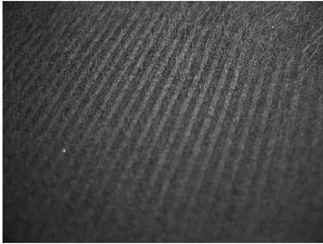
Fig. 6. Picture of a PTL showing localized compression under the land area [17] (dark striations correspond to PTL under the land area that have been subjected to compression).
